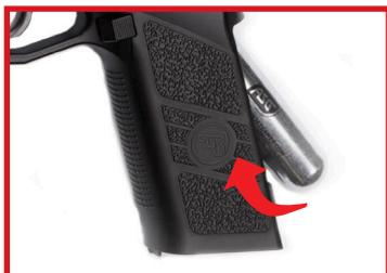
Load the 12g CO<sub>2</sub> capsule into the CO<sub>2</sub> compartment.
