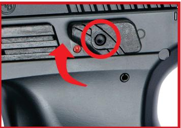
To unlock the safety, press the button as indicated and push the safety lever upwards. With the red dot visible, the Airgun is ready to fire.
